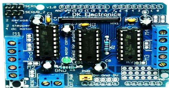
**Fig. 7: Adafruit Motor Shield**
